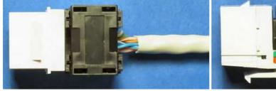
Note: Avoid bending the cable sharply at the point of entry when the keystone jack is snapped into place.
