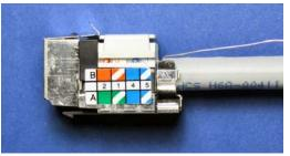
8 Wrap the drain wire around the cable under the metal ribs and strap the cable with the ribs tightly using a tie wrap (included).
