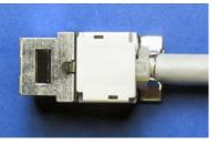
9 Slide the metal shield into place, close the back cover and fold the fin properly.
