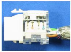
11 Make sure the two grounding belts are inserted into the two slots.
