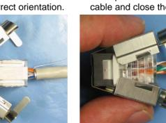
13 Wrap the ground wire and press tightly both grounding belts.
