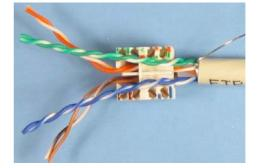
**5** Cut the wires flush with a sharp tool.
