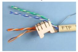
4 Insert the wires into the correct colored slots.
