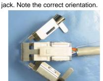
12 Pull the grounding belts with a suitable pliers and fold them.
