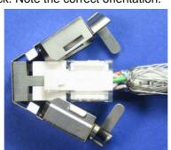
12 Pull the grounding belts with a suitable pliers and fold them.
