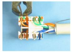
6 Slide the wiring block into the the jack housing with the colored side down and push gently with your thumb. Note the guide and the IDC contacts.
