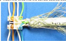
6 Slide the wiring block into the the jack housing with the colored side down and
