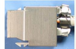
Note: Avoid damaging the cable when using the pliers and make sure the drain wire is in good contact with the keystone jack shield.
