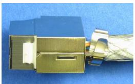
Note: Avoid damaging the cable when using the pliers and make sure the braid shield is in good contact with the keystone jack shield.
