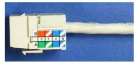
Note: Avoid bending the cable sharply at the point of entry when the keystone jack is snapped into place.
