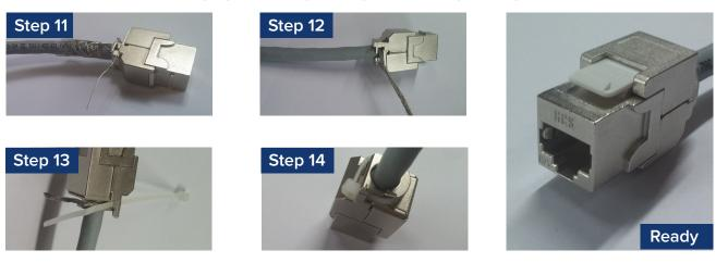
Note: Avoid damaging the cable when using the pliers and make sure the braid shield is in good contact with the keystone jack shield.
