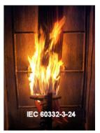
Metal foil shields in LAN cables (F/UTP, U/FTP or S/FTP) act also as partial flame retardants, but in U/UTP LS0H cables the plastic materials are fully exposed to the flames, so these cables must have special design and they must be made from special plastic materials.
